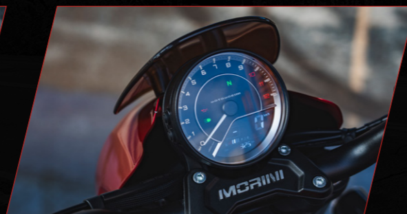
Digital display integrated into the analog dashboard
